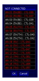
If the desired input pinout is currently allocated then it will be displayed in RED. The WHITE items show free spaces
