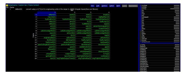
In the unlikely event that the Gauges are displaying the wrong values on the App. Head to the Custom Stream Config under the Settings tab. Here you are able to change the Stream Config to match your Syvecs output stream.
